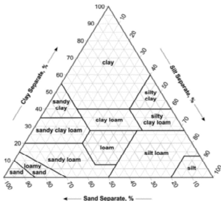
Figure 1. Soil Texture Depending on Percentages of Sand, Silt and Clay (Source: USDA Natural Resource Conservation Service).
